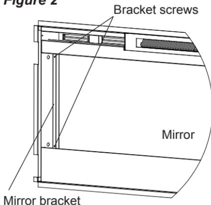
fireplace upright and slightly forward to allow the mirror to fall out of the inside framing.
